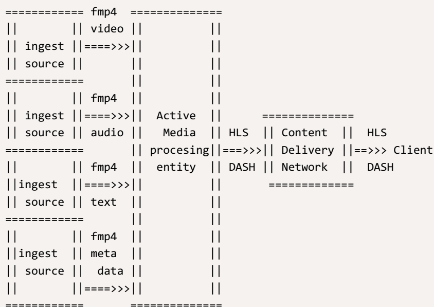
Diagram 7: fragmented MPEG-4 ingest with multiple ingest sources
