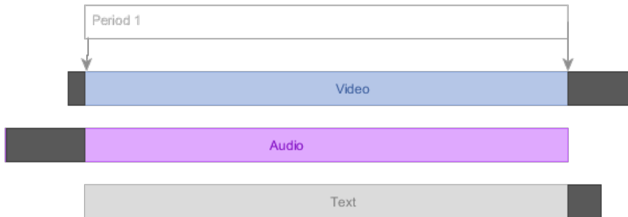
Figure 23 Content may be cut (indicated in black) to equalize track lengths.
