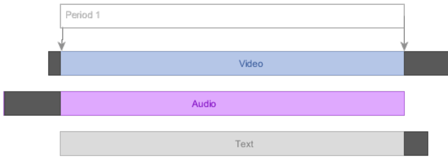
Figure 20 Content may be cut (indicated in black) to equalize track lengths.
