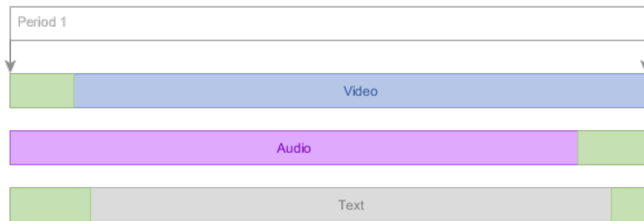
Figure 21 Content may be padded (indicated in green) to equalize track lengths.
