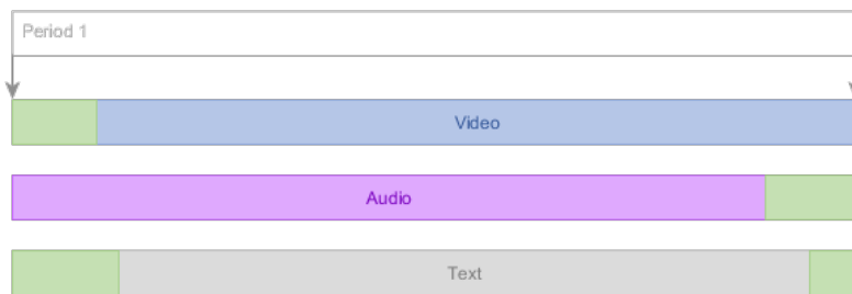
Figure 20 Content may be padded (indicated in green) to equalize track lengths.
