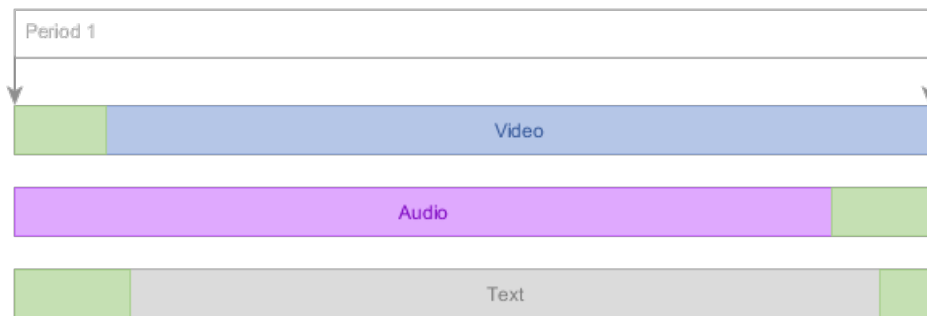
Figure 22 Content may be padded (indicated in green) to equalize track lengths.
