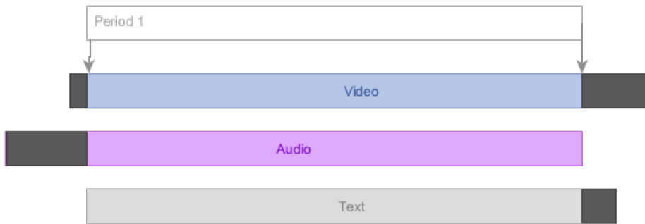
Figure 21 Content may be cut (indicated in black) to equalize track lengths.
